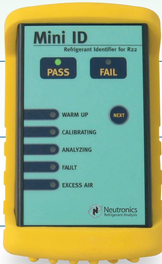
Easy to use with 'PASS' or 'FAIL' result indication for system under test
